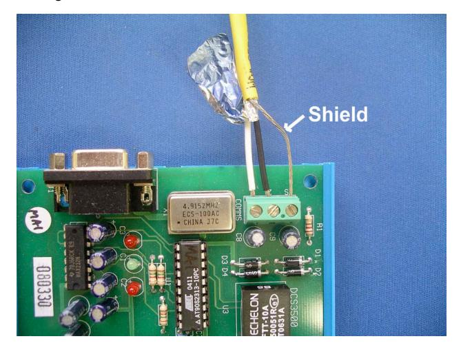
Ensure the shield wire is connected to the terminal marked S
