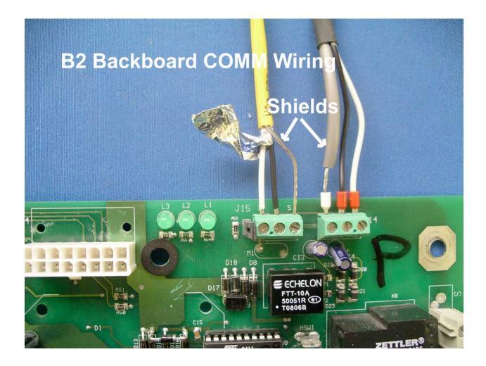
Shields must be connected to the terminals marked S
